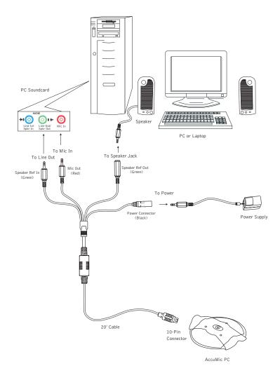
Figure 6. AccuMic PC connections
